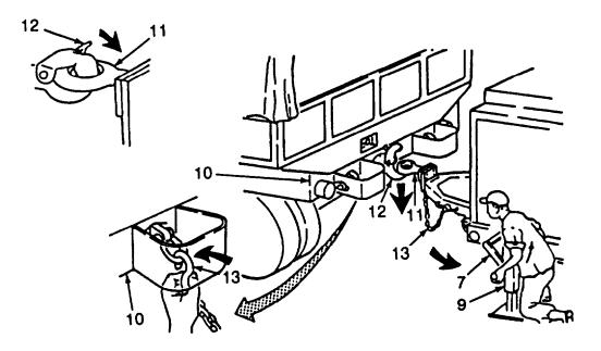
4. PLACE CRANK HANDLE (7) ON FRONT JACK (9). SLOWLY BACK TOWING VEHICLE (10) INTO POSITION SO THAT LUNETTE (11) ALIGNS WITH PINTLE (12). RAISE OR LOWER FRONT OF TRAILER AS NECESSARY TO POSITION LUNETTE (11) IN PINTLE (12). CLOSE PINTLE (12).
