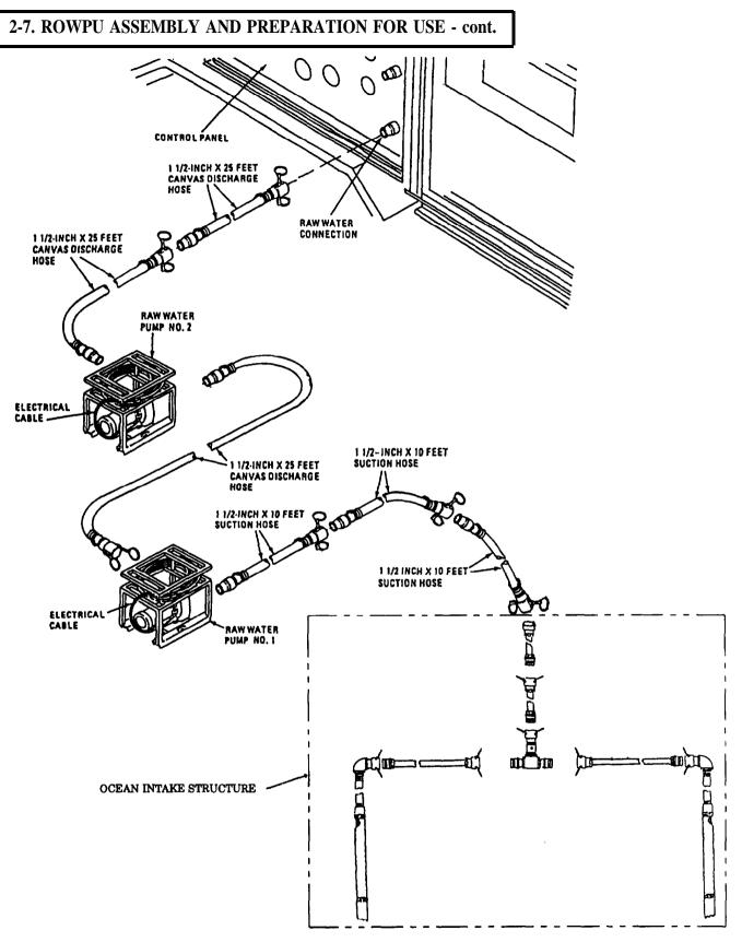
Figure 2-36b. Setup of Raw Water System Using Ocean Intake Structure.
