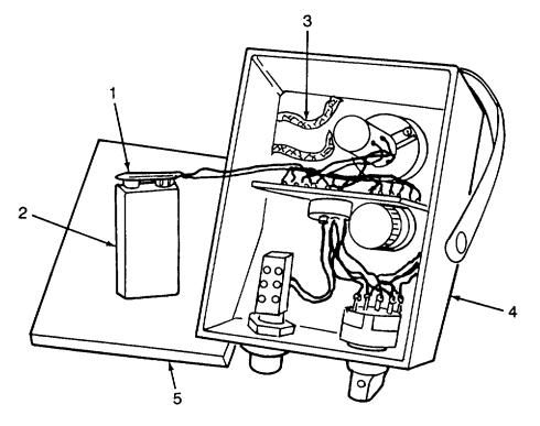
Figure 3-8. TDS Meter Battery Replacement.
