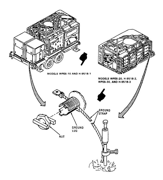
Figure 2-43. Ground Strap Installation (Sheet 2 of 2).
