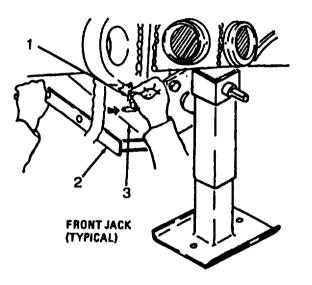
12. POSITIONCRANK HANDLE (12) ON JACK (14) AND TURN HANDLE COUNTERCLOCKWISE TO RETRACT JACK UNTIL JACK PAD (15) 15 CLEAR OF SECUREMENT PLATE (16) ROUND BAR.
