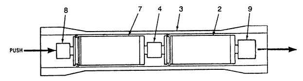
Figure 3-5. R.O. Element Installation
