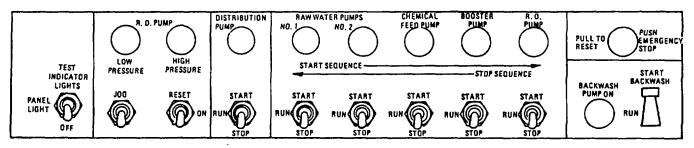
Figure 2-48. Control Box Switches.
