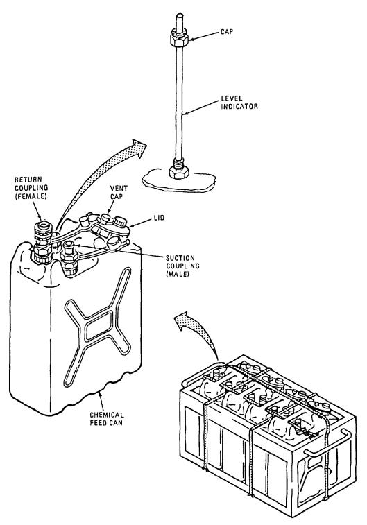
Figure 2-41. Chemical Feed Can Indicator.
