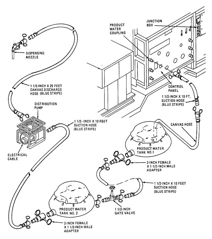
Figure 2-38. Product Water System Setup.
