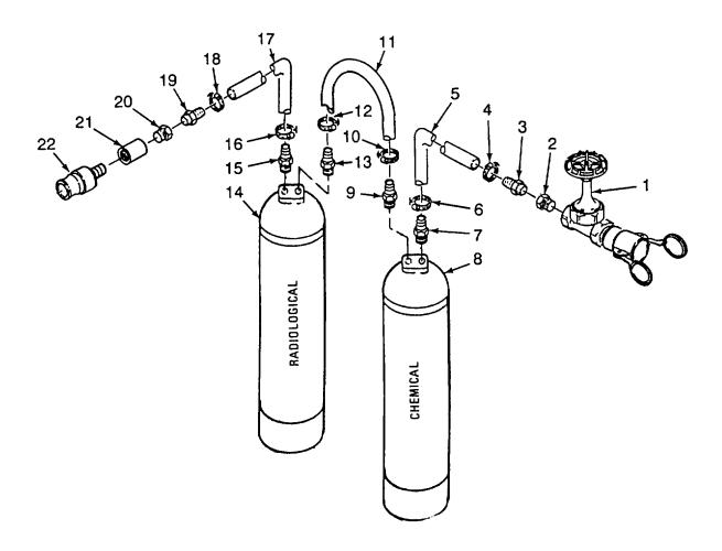
Figure 2-79. Nuclear, Biological and Chemical Filter System Assembly.
