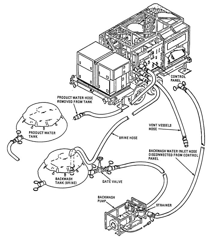
Figure 2-69. Citric Acid Element Cleaning.
