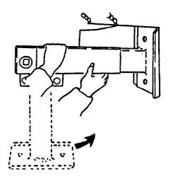
9. TO ROTATE FRONT LEVELING JACK TO HORIZONTAL POSITION, REMOVE CRANK HANDLE, GRASP JACK AND PULL STRAIGHT OUT AGAINST SPRING TENSION. ROTATE JACK UP TO HORIZONTAL POSITION. ALLOW JACK TO SPRING BACK TO COCKED POSITION.
