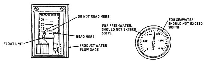
Figure 2-73. Product Water Flow Adjustment.
