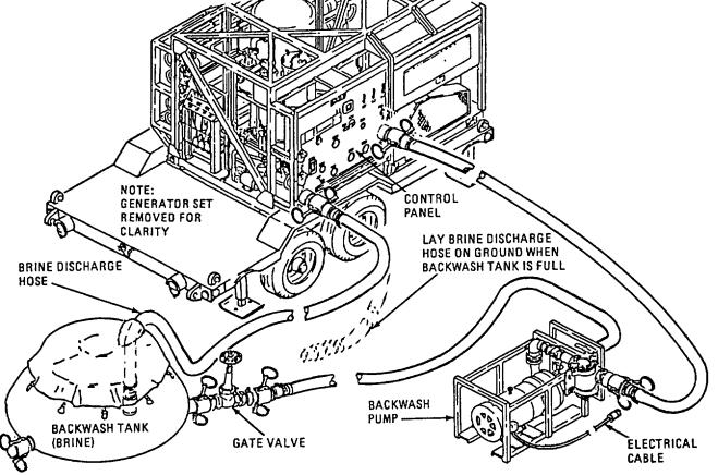
Figure 2-62. Fill Backwash Tank.
