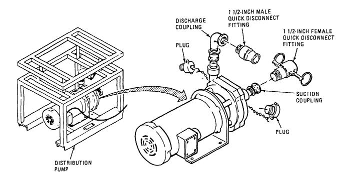
Figure 2-29. Distribution Pump Quick Disconnect Fittings.
