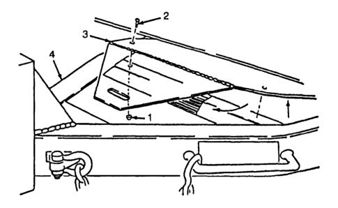
1. REMOVE NUTS (1) AND SCREWS (2) SECURING SAFETY STEP IN PLACE. LIFT STEP UP AND FOLD END PLATE (3) UNDER PLATE (4). LAY BOTH PLATES BACK DOWN AND FASTEN BOTH TO TRAILER DRAWBAR (5) WITH SECURING NUTS (1) AND SCREWS (2).
