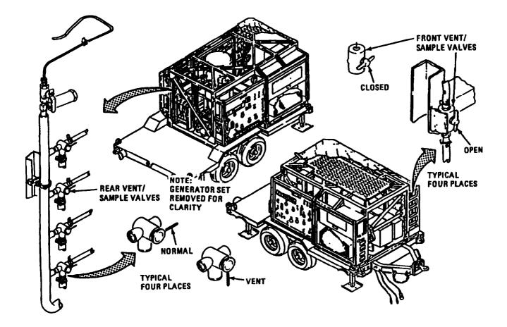
Figure 2-47. R.O. Tube Vent/Sample Valves.
