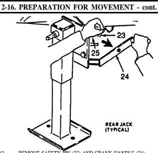
12. REMOVE SAFETY PIN (23) AND CRANK HANDLE (24) FROM REAR OF JACK SUPPORT BRACKET (25).
