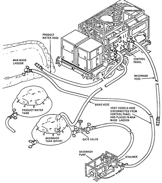
Figure 2-70. Rinsing Citric Acid From Backwash Tank.
