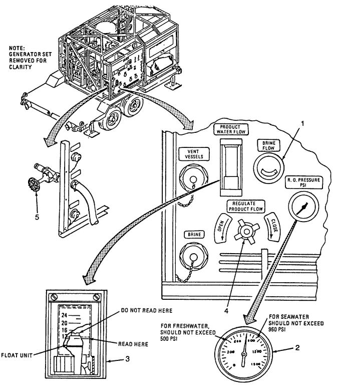
Figure 2-61. Final Adjustments
