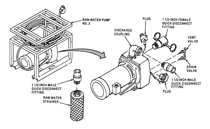
Figure 2-27. Raw Water Pump No. 2 Quick Disconnect Fittings.
