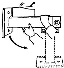
15. REPLACE CRANK HANDLE (12) ON REAR OF JACK SUPPORT BRACKET (13); INSTALL SAFETY PIN (11).  POSITION CRANK HANDLE (12) ON JACK (14) AND TURN HANDLE CLOCKWISE TO LOWER JACK PAD (15).
