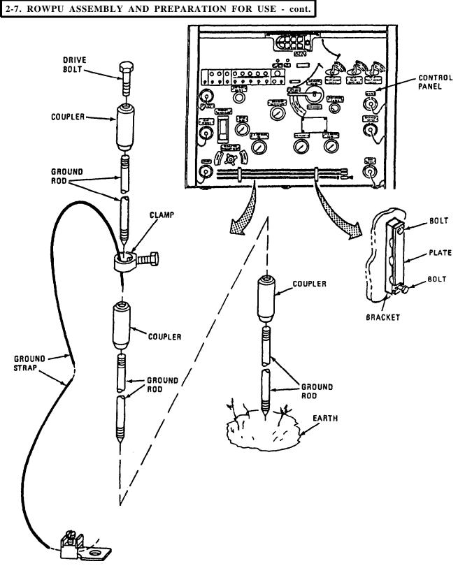
Figure 2-43. Ground Rod Installation (Sheet 1 of 2).
