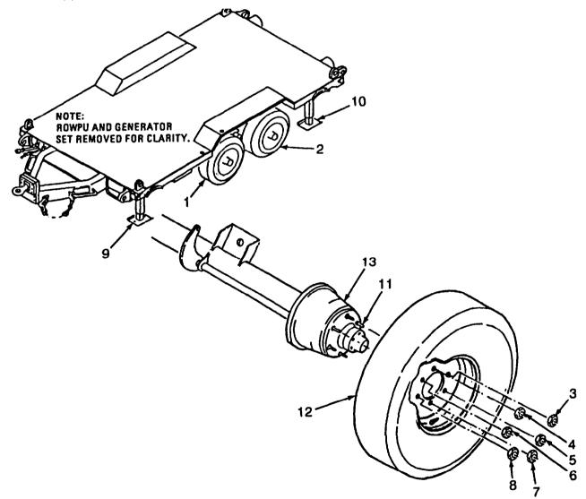
Figure 3-14. Tire and Wheel Replacement.
