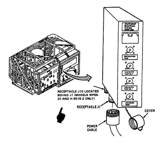
Figure 2-44. Power Cable Connection.
