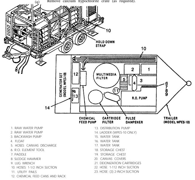
Figure 2-24. ROWPU Accessory Overpack (sheet 1 of 2).
