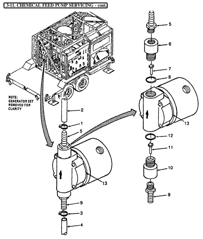
Figure 3-13. Chemical Feed Pump Assembly.
