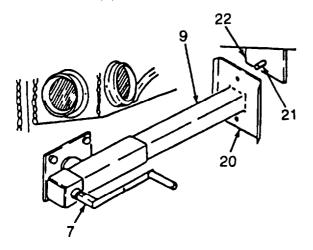
10. POSITION CRANK HANDLE (7) ON FRONT JACK (9) AND TURN HANDLE CLOCKWISE TO EXTEND JACK PAD (20). LINE UP HOLES IN JACK PAD WITH ROUND BAR (2) ON SECUREMENT PLATE (22). EXTEND JACK UNTIL JACK PAD RESTS FIRMLY AGAINST SECUREMENT PLATE.
