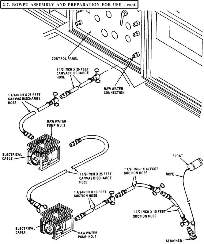
Figure 2-36. Raw Water System Setup.
