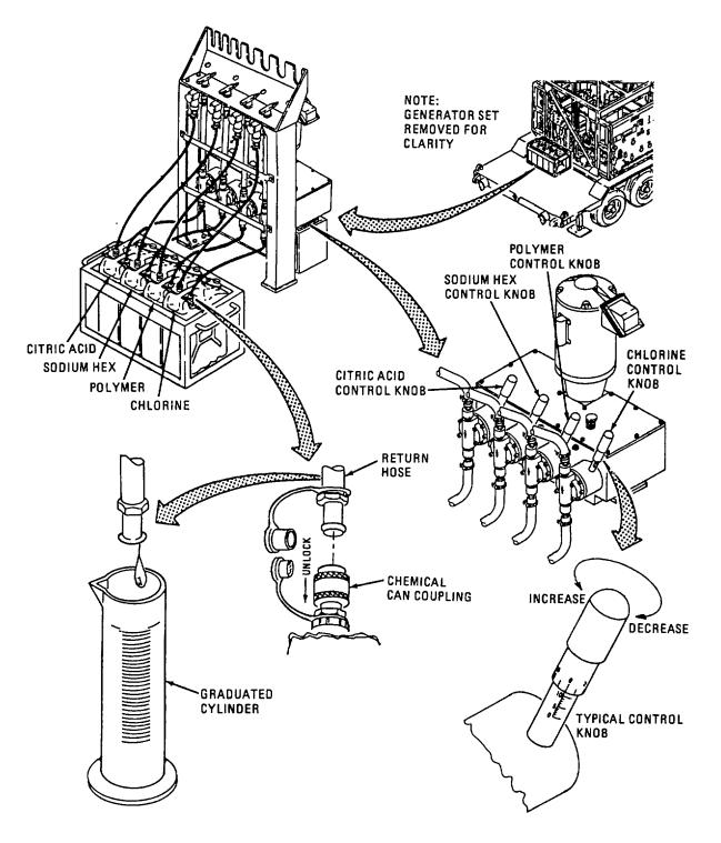
Figure 2-56. Chemical Feed Pump Adjustment.
