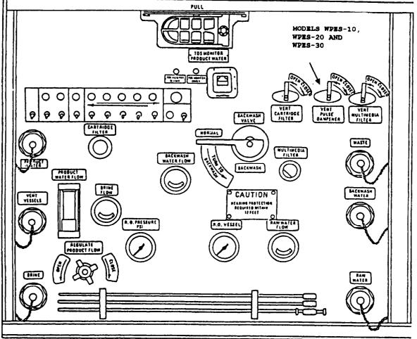
Figure 2-76. Decals and Instruction Plates (sheet 2 of 6).
