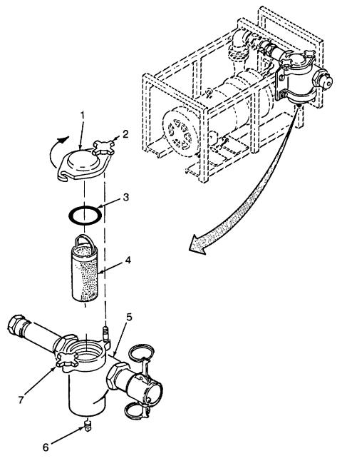
Figure 3-7. Backwash Pump Strainer Cleaning.
