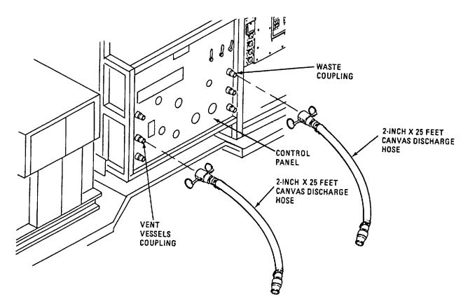
Figure 2-39. Waste Water System Setup.
