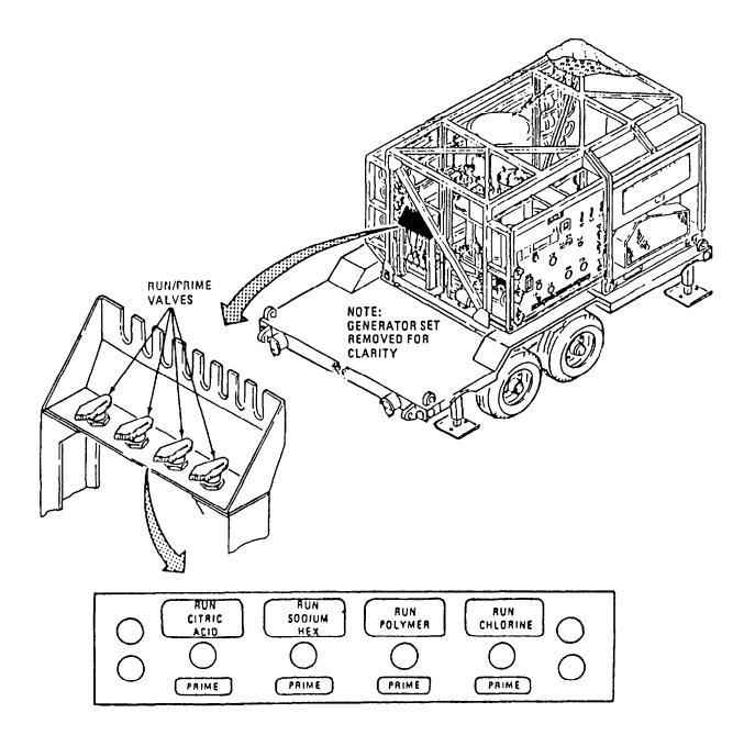
Figure 2-11. Chemical Feed Run/Prime Valves.
