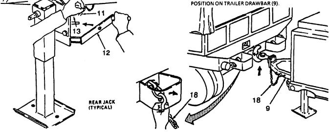
Figure 2-19. Trailer Preparation for Use (Sheet 4 of 5) (Models WPES-10 and H-9518-1) 2-6. TRAILER ASSEMBLY AND PREPARATION FOR USE (Models WPES-10 and H-95181) - cont.
