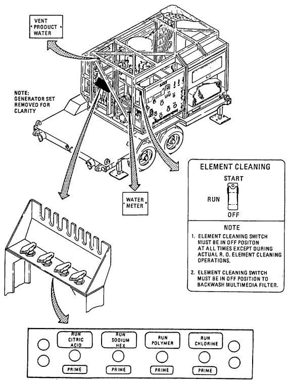
Figure 2-76. Decals and Instruction Plates (sheet 4 of 6).
