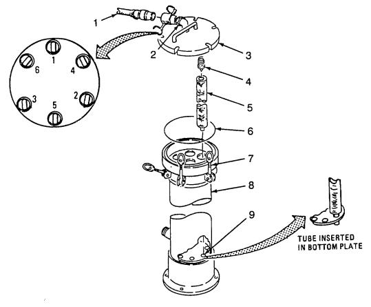
Figure 3-6. Cartridge Filter Tube Replacement.
