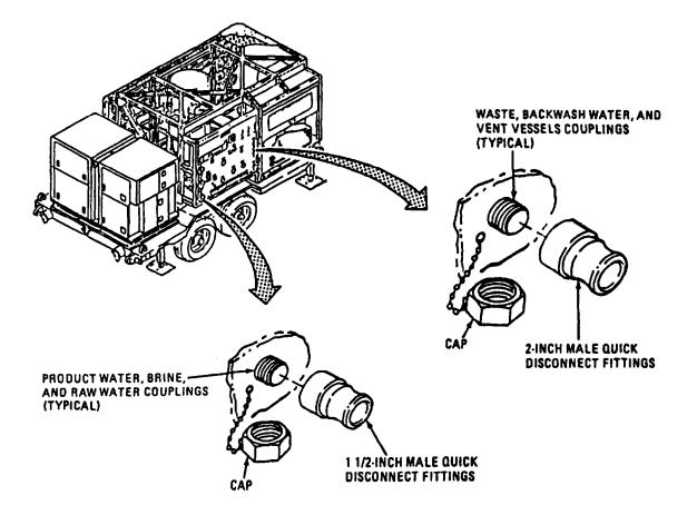
Figure 2-25. Control Panel Quick Disconnect Fittings.
