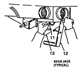
10. REPLACE CRANK HANDLE (2) ON REAR OF JACK SUPPORT BRACKET (3); INSTALL SAFETY PIN (1).
