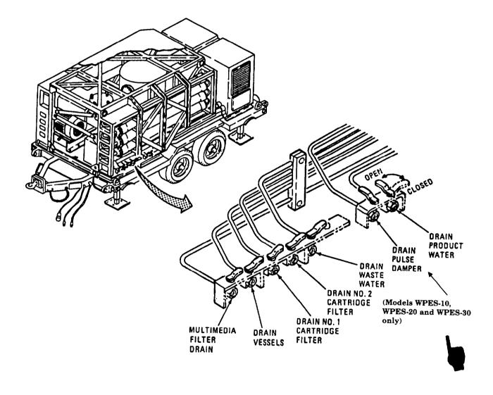
Figure 2-45. Drain Valves
