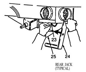
16. REPLACE CRANK HANDLE (24) ON REAR OF JACK SUPPORT BRACKET (25); INSTALL SAFETY PIN (23)
