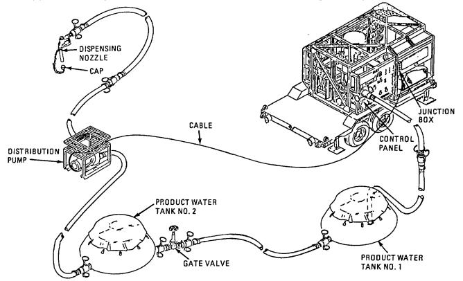
Figure 2-63. Filling Product Water Tanks.
