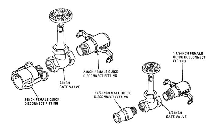
Figure 2-31. Gate Valve Quick Disconnect Fittings.
