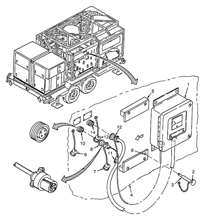
Figure 2-33. TDS Monitor Installation.
