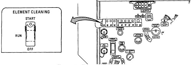
Figure 2-49. Element Cleaning Switch.
