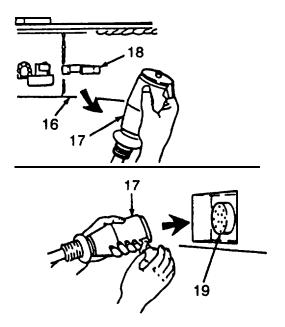
7. REMOVE ELECTRICAL CONNECTOR (17) FROM STOWAGE CLIP (18) ON TRAILER DRAWBAR (16) AND CONNECT IT TO MATING RECEPTACLE (19) ON TOWING VEHICLE.
