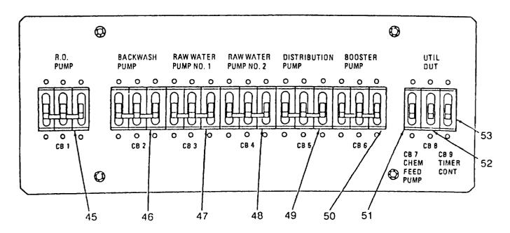
Figure 2-5. ROWPU Controls and Indicators (sheet 3 of 3).
