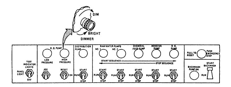
Figure 2-53. Control Box Emergency Stop Button, Switches and Lamps.
