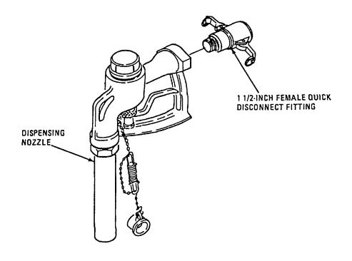
Figure 2-30. Dispensing Nozzle Quick Disconnect Fittings.
