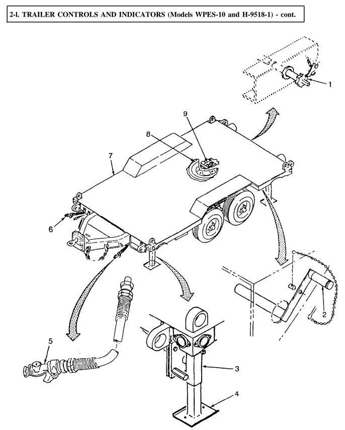
Figure 2-3. Trailer Controls and Indicators.
