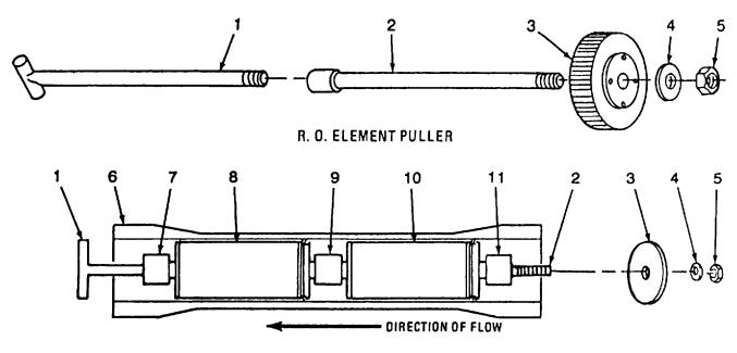
**INSTALLING R. O' ELEMENT TOOL**
