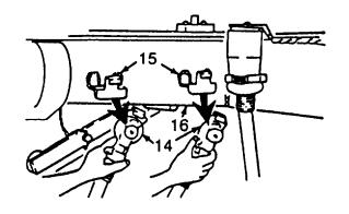
6. REMOVE AIR HOSES (14) FROM DUMMY COUPLINGS (15) ON TRAILER DRAWBAR (16) AND CONNECT TO TOWING VEHICLE.
