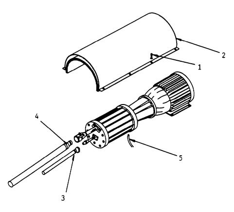
Figure 2-76a. Draining of R.O. Pump (Models H-9518-1, H-9519-2, and H-9518-3)
