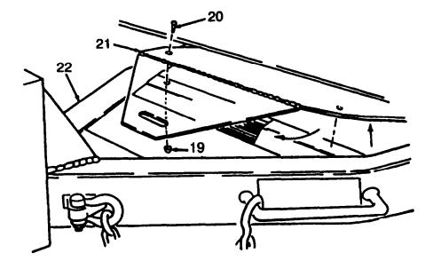
17. REMOVE NUTS (19) AND SCREWS (20) SECURING SAFETY STEP (21) IN PLACE. LAY SAFETY STEP DOWN ON DRAWBAR (22) AND INSTALL PREVIOUSLY REMOVED NUTS AND SCREWS.
