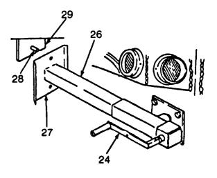
15. POSITION CRANK HANDLE (24) ON REAR JACK (26) AND TURN HANDLE CLOCKWISE TO EXTEND JACK PAD (27). LINE UP HOLE IN JACK PAD WITH ROUND BAR (28) ON SECUREMENT PLATE (29). EXTEND JACK UNTIL JACK PAD RESTS FIRMLY AGAINST SECUREMENT PLATE.
