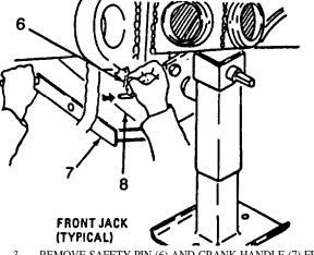
3. REMOVE SAFETY PIN (6) AND CRANK HANDLE (7) FROM REAR OF JACK SUPPORT BRACKET (8).
