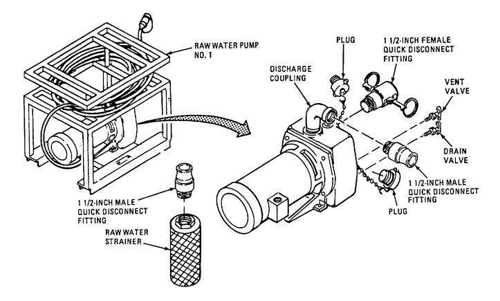
Figure 2-26. Raw Water Pump No. 1 Quick Disconnect Fittings.
