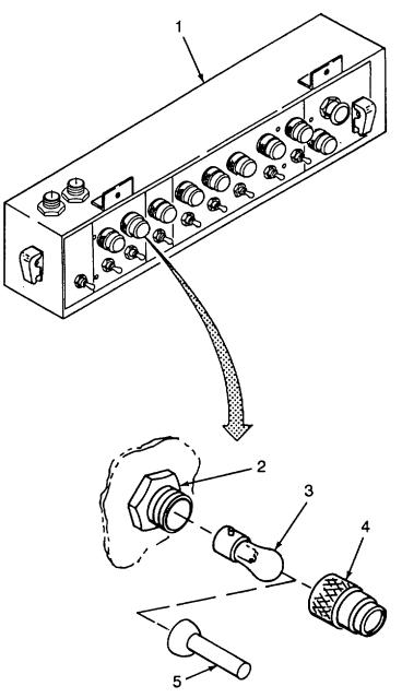
Figure 3-9. Switch Indicator Lamp Replacement.
