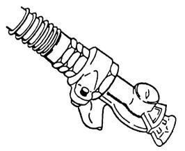
Figure 2-1. Trailer Electrical Plug.
