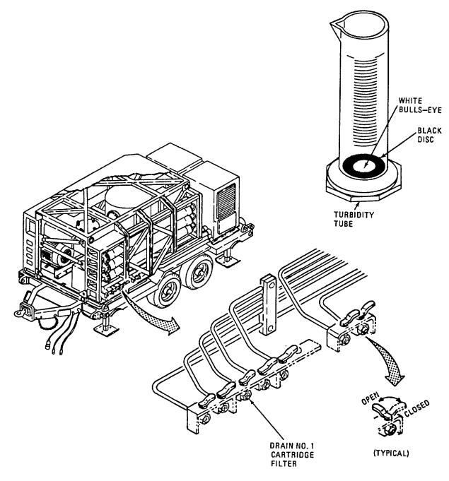
Figure 2-59. Drain Valves and Turbidity Tube.
