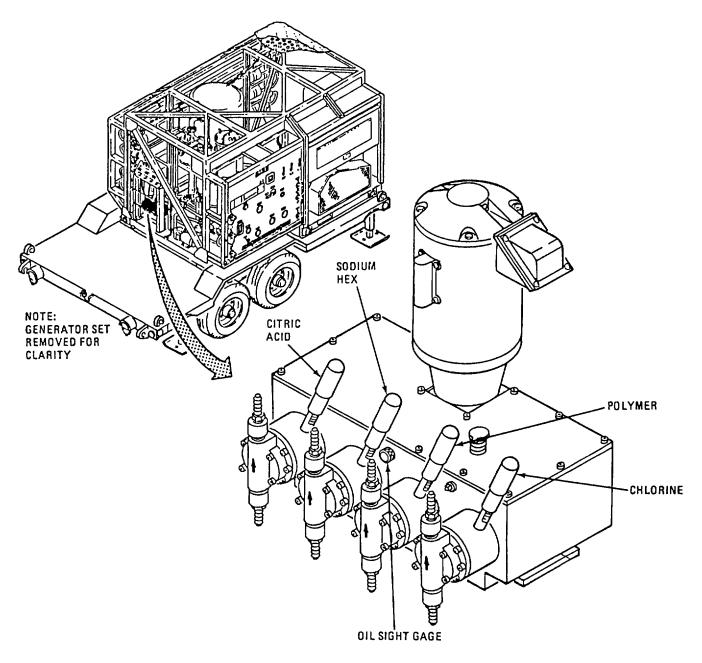
Figure 2-8. Chemical Feed Pump Controls and Indicator.
