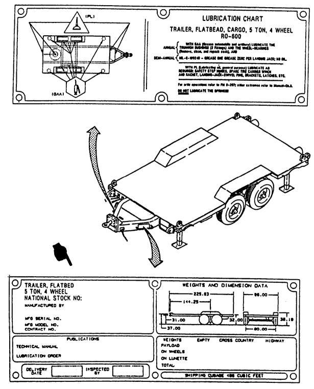
Figure 2-76. Decals and Instruction Plates (sheet 6 of 6).
