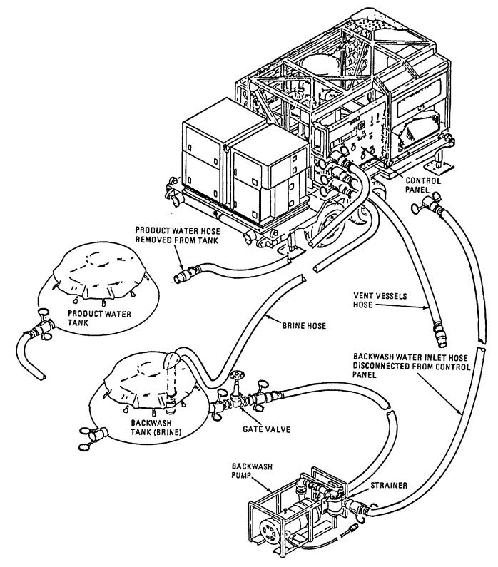
Figure 2-67. Lowering Water Level in Backwash Tank
