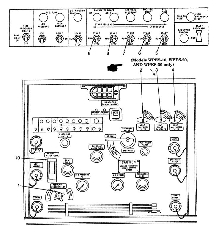
Figure 2-74. Shutdown Position of Control Panel Switches and Valves.
