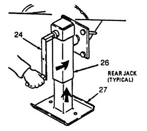
13. POSITION CRANK HANDLE (24) ON REAR JACK (26) AND TURN HANDLE COUNTERCLOCKWISE TO RAISE JACK PAD (27).
