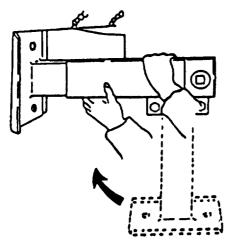
14. TO ROTATE REAR LEVELING JACK TO HORIZONTAL POSITION, REMOVE CRANK HANDLE, GRASP JACK AND PULL STRAIGHT OUT AGAINST SPRING TENSION. ROTATE JACK UP TO HORIZONTAL POSITION. ALLOW JACK TO SPRING BACK TO LOCKED POSITION.
