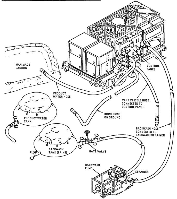
Figure 2-71. Rinsing R.O. Pressure Tubes.
