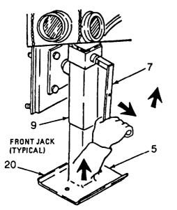
8. WITH CRANK HANDLE (7) IN POSITION ON FRONT JACK (9), TURN CRANK HANDLE COUNTERCLOCKWISE AND FULLY RAISE JACK PAD (20)
