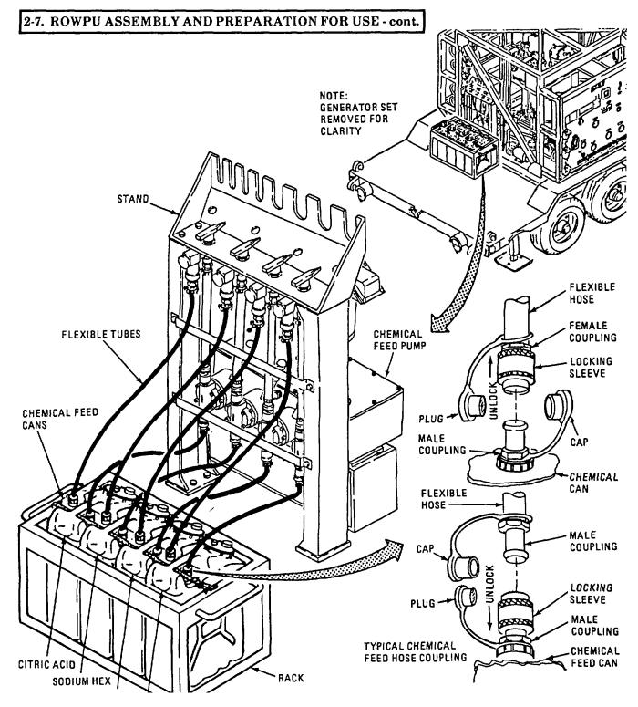
Figure 2-42. Chemical Feed Can Connections.
