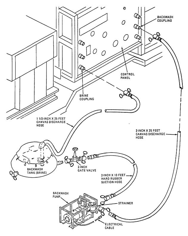
Figure 2-37. Backwash System Setup.
