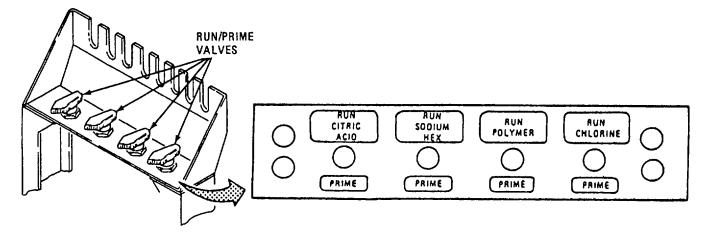
Figure 2-50. Chemical Feed Run/Prime Valves.
