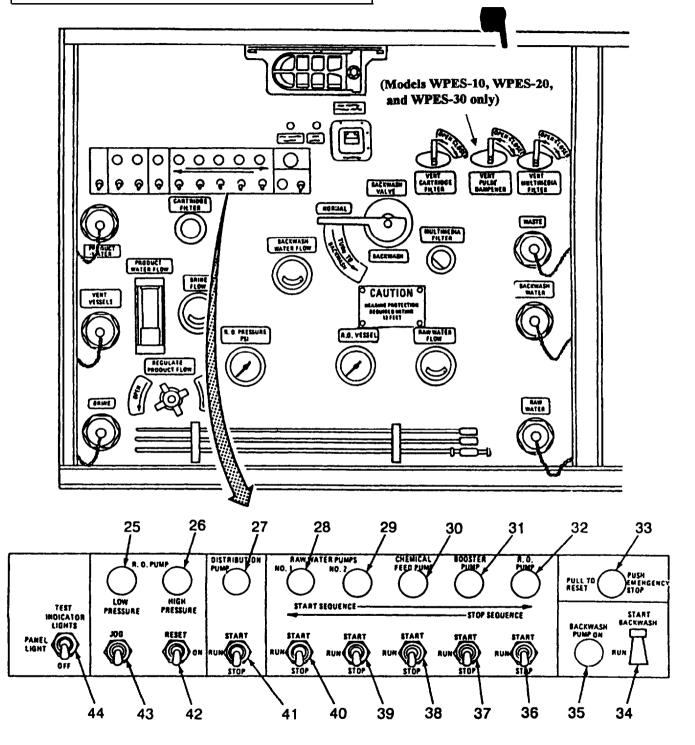
Figure 2-5. ROWPU Controls and Indicators (sheet 2 of 3)
