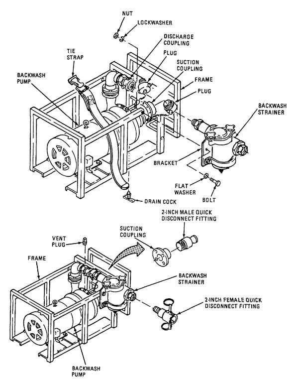
Figure 2-28. Backwash Pump Quick Disconnect Fittings.
